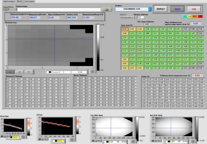
Following laser measurement, the sample passes through an x-ray scanner and the raw x-ray image data obtained, is subjected to complex image processing algorithms resulting in coloured density mapping of the sample. As shown here, internal defects and density measurement can be further quantified using the software functions (as shown here on the right-hand side).
