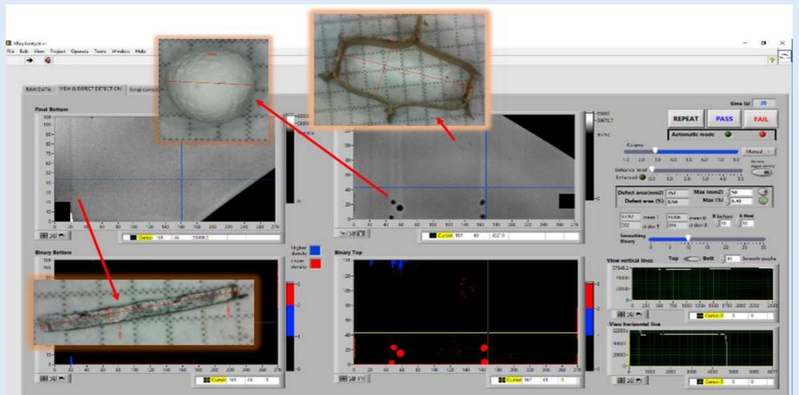
The XShaper laser measurement software provides a 3D profile of the specimen and calculates volume, surface area and overall density, it maps the thickness over the full surface area and records a matrix of 110 point thickness readings, which is then used for comparative coloured thickness mapping.
